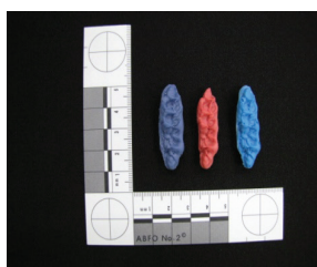
Figura 3c: Chewing gum replication using silicone (left side) and vinyl polysiloxane material (right side), and the original chewing gum (middle).
