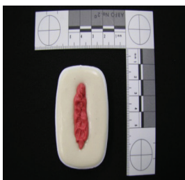
Figure 2b: chewing gum included in the plastic recipient containing alginate
