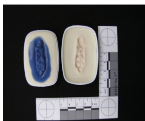
Figura 3b: Chewing gum replication after material cure; notice that the excess material must be removed
