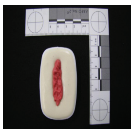
Figure 2b: chewing gum included in the plastic recipient containing alginate
