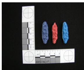
Figura 3c: Chewing gum replication using silicone (left side) and vinyl polysiloxane material (right side), and the original chewing gum (middle).
